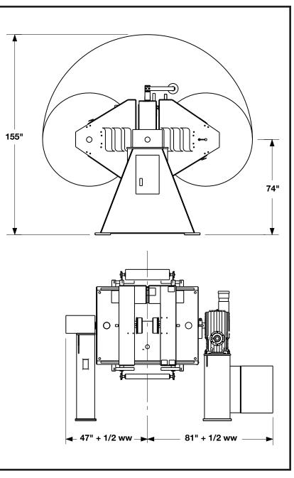
Footprint dimensions will depend on roll diameter and web width. Dimensions shown are for 72 inch diameter, 6000 lb roll. Call Martin with your process specifications.
