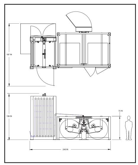
Dimensions shown are for an 1500 FPM 65 IN web-width machine
