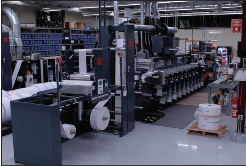
MBS butt splicer on a Gallus press. All art courtesy of Martin Automatic.
